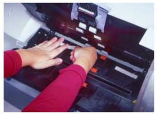
8. Lower the scanner door and press it firmly until it snaps into place.
